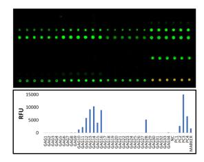
scanned with InnoScan 710 microarray scanner (XDR mode) at 1 PMT and 100% laser power at 532nm wavelength. The positive control 3 (mouse IgG) shows binding as expected.
